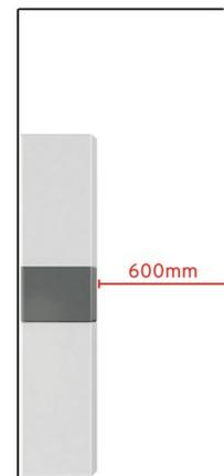
If the gap between the top of the inverter and the ceiling is less than 600mm, the ceiling and any wall within a 600mm radius must be made of non-combustible material.
