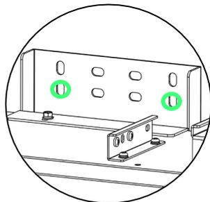
**Option 2: If you are installing a 10.2kWh system (2 batteries) AND this is the first of the two**
